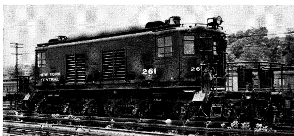
Class T type of electric locomotive of the New York Central railroad
