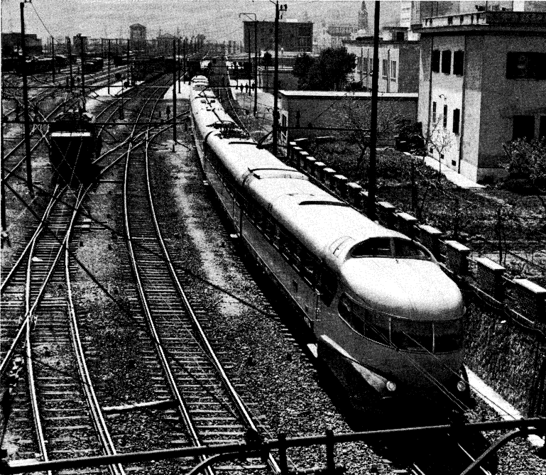
ETR 300 "Settebello," a high-speed electric passenger train of the Italian State railways. Unique design provides passengers with an observation area in the first car while the engineer operates the train in a "blister" cabin above
