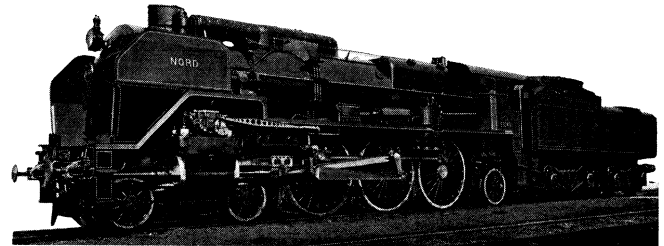
Pacific (4-6-2) of the French railways, typical locomotive of the years between World War I and World War II
