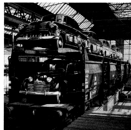
German automobile carrier, a two-decked, five-axle type which will hold 10 compact cars
