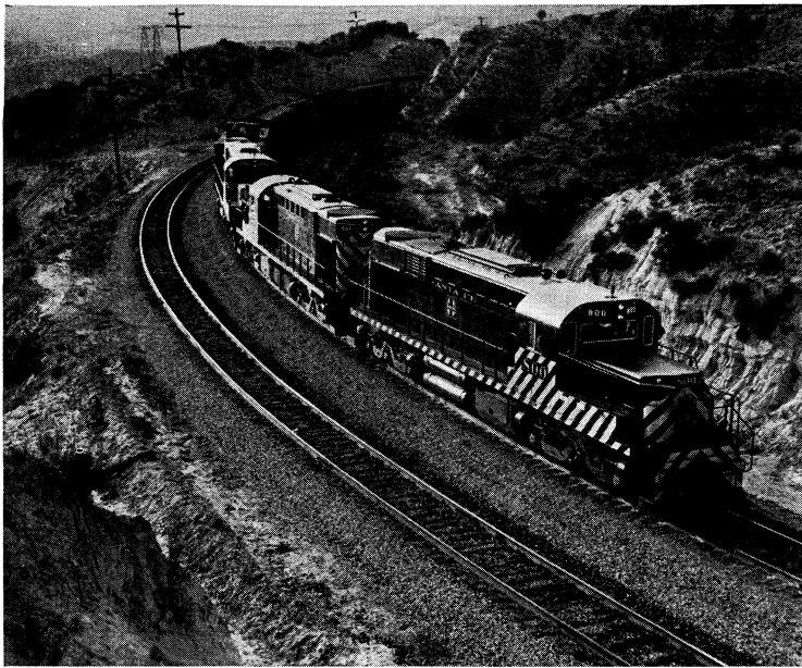
Three DL-600 locomotives, 2,400-h.p. modern diesel-electric units powered by 16-cylinder engines. Sante Fe, U.S.
