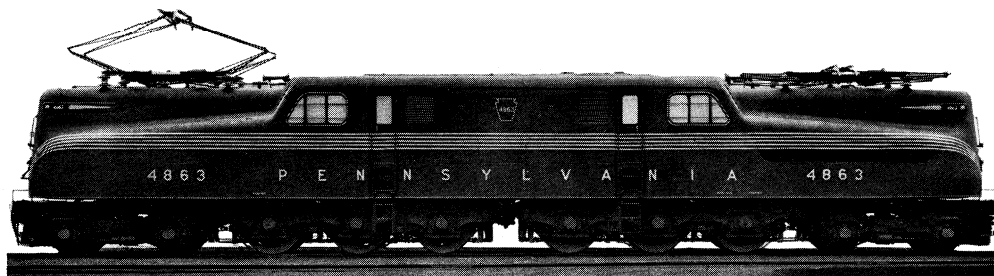
Pennsylvania railroad (U.S.) GG-1, a 2-C+2-C electric used for high-speed passenger and freight operations
