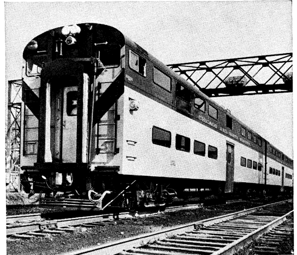
Double-deck coach for commuters on the suburban divisions of the Chicago and North Western railway
